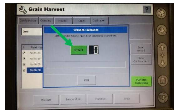
4. After timer expires, the system will make calculations and will inform you when calibration is completed. Throttle down and disengage. Press the Exit to complete calibration.
