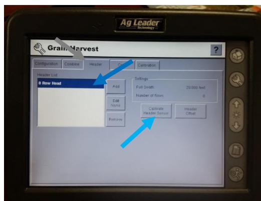
3. Read the message on the screen and then press the **Next button**. Raise the header all the way up, press **Set Max**. Next, lower the header all the way down, press **Set Min**. This only needs to be completed once per combine. **Press Next** to continue.
