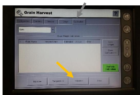
3. To begin calibration, start the separator and engage the header, increase engine speed to full throttle and press **START**.
