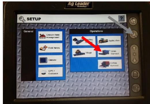
2. Press on the **Header Tab**. Touch the head that is currently on the machine to highlight it. With the **head highlighted**, press the **Calibrate Header Height** button.
