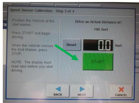
4. Measure and mark out a distance greater than 100 ft., 300ft recommended. Change "Actual Distance" to match measured distance. Press Continue. Press **START** and begin driving marked distance. At the end of the track, press **STOP**. Press the **Next** then the **Green Checkmark** to complete calibration.
