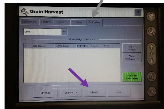
**NOTE:** The temperature calibration should be performed in the early morning (or in the shade) before the combine has been running, to avoid heat from the machine affecting the reading. This calibration only needs to be completed once per season.
