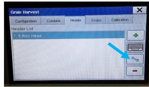
3. Press the **Calibrate Header Sensor** Button. Read the message on the screen and then press the **Blue Right Arrow**.
