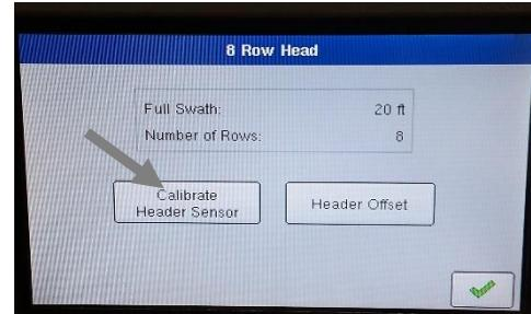
4. Raise the header all the way up, press **Set Max**. Next, lower the header all the way down, press **Set Min**. This only needs to be completed once per combine. **Blue Right Arrow** to continue.
