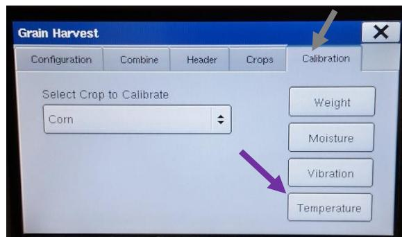
3. Adjust the temperature using **Up and Down Arrows** to match ambient outdoor temperature. Press the **Green Checkmark** to complete the calibration.
