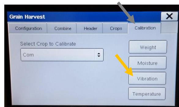
3. To begin calibration, start the separator and engage the header, increase engine speed to full throttle and press **START**.
