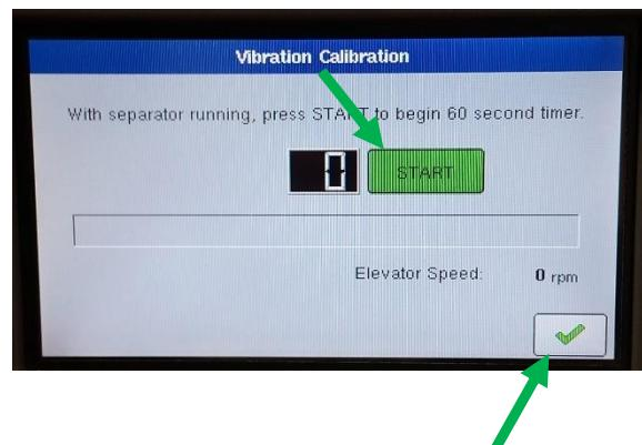
4. After timer expires, the system will make calculations and will inform you when calibration is completed. Throttle down and disengage. Press the **Green Checkmark** to complete the calibration.
