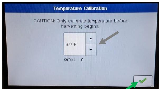
**NOTE:** The temperature calibration should be performed in the early morning (or in the shade) before the combine has been running, to avoid heat from the machine affecting the reading. This calibration only needs to be completed once per season.
