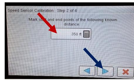
6. Press Continue. Press **START** and begin driving marked distance. At the end of the track, press **STOP**. Press the **Next** then the **Green Checkmark** to complete calibration.
