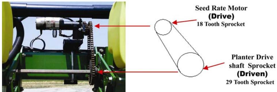
$$\frac{\text{\# Of Teeth on the (Driven) Sprocket}}{\text{\# Of Teeth on the (Drive) Sprocket}} = \text{Gear Ratio}$$
