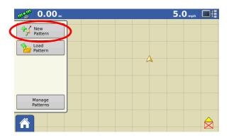
Using the Change Pattern Button, select the desired guidance pattern. Double check that the proper Guidance Width is entered on the right (changes can be made by pressing the Calculator Button). Press the Green Checkmark to accept your selections.
