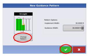
Press the A-B Button to set your A Point, drive the desired distance and press the A-B Button again to set the B Point.
