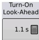
**Turn-On Look-Ahead** This option determines how far ahead of time (in seconds) the system must engage the clutch before entering a planted area. Note: this value is in seconds. For best performance, do not change travel speed as you are nearing the planted area. Accelerate either well before entering the planted area, or after all clutch sections have turned on.
