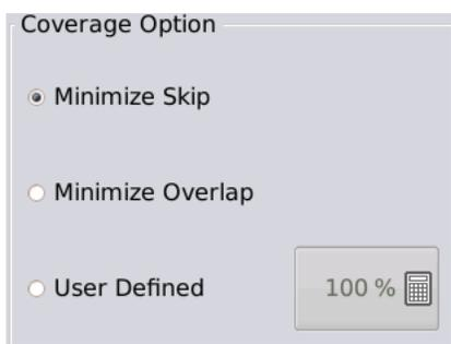
**Minimize Skip** - The entire clutch section rectangle (shown to the right) must pass into non planted area before the section will cease planting.
