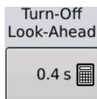
**Turn-Off Look-Ahead** How far ahead of time (in seconds) the system must disengage the clutch before exiting a planted area. Note: this value is in seconds. For best performance, do not change travel speed as you are exiting the planted area, wait until clutch sections have turned off
