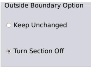
**Keep Unchanged** - Clutch section on/off status will not change when exiting the field as defined by the outside boundary.
