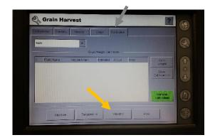
After timer expires, the system will make calculations and will inform you when calibration is completed. Throttle down and disengage. Press the Exit to complete calibration.
